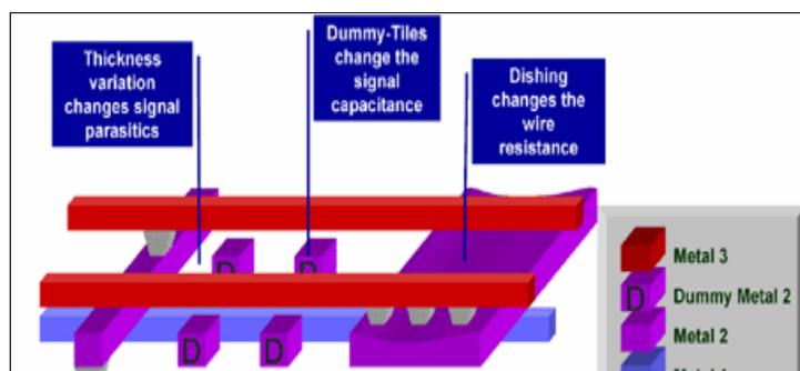
and even functionality. Tight control of planarity requires dummy tiles to be placed in close proximity to functional features. This may cause coupling with functional wires – and creates additional parasitics. The existence of the tiles changes capacitance. CMP dishing changes wire resistance, and dielectric thickness variations also change signal parasitics. Originally, this planarization was a yield enhancement technique today, however, CMP can pose a yield challenge.
