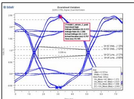
SI / timing analysis results can be displayed as scatter plots, showing how voltage and timing margins are distributed across an interface. Waveform quality violations can be highlighted on screen and examined in detail.
