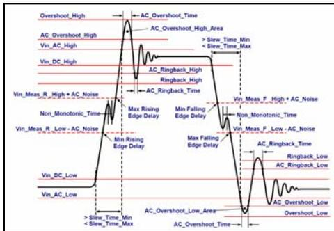
The Quantum-SI timing analysis engine combines interconnect delays with component timing data to provide an integrated signal integrity and timing report. This report includes summary data for waveform quality and timing margins, accompanied by multiple levels of drill-down detail.
