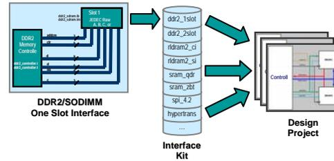
Quantum-SI design kits can shave weeks to months off your next project by reducing model development and interface capture efforts. Design kits include validated timing and signal integrity models, transfer net topologies and analysis settings for standard interface technologies including DDR2, DDR3, QDR SRAM, RLDRAM, PCI-Express, SATA, USB2 and XAUI.
